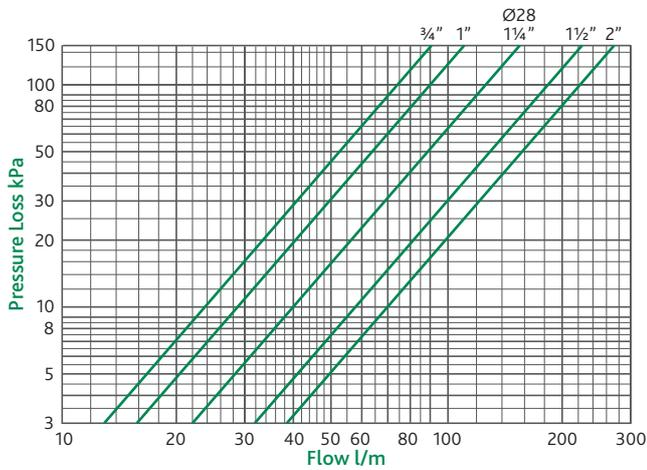
Flow rates recommended to ensure stable operation and accuracy of  $\pm 2^\circ\text{C}$  (balanced pressure Hot/Cold)
